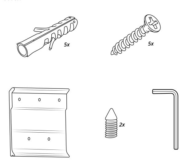
**Please note:** the shower seat should be secured to a flat, solid wall (brick or concrete block) and away from cavities, voids, cables and pipes when locating the fixing screws.
