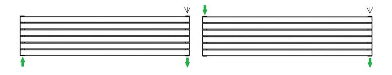
• This product can only be used at PN 1MPa (10g/cm², 10 Bar). It should only be filled with water, and at a temperature below 100 °C (212°F). See table below for installation requirements.
