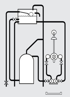
Unvented Mains Pressure Showers The shower valve can be used on an unvented mains pressure system. This type of system must only be installed by a competent person as per the requirement of Part G of Schedule 1 to the building regulations.
