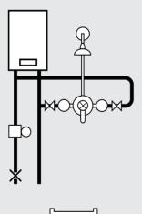
Gas Heated/Combi-Boiler Showers The shower valve must be installed with a modulating type combi-boiler or multipoint gas water heater. This system will produce a constant flow of water within the operating specifications of the appliance. NB The outlet temperature of the system must be capable of supplying hot water in excess of 100.4°F.
